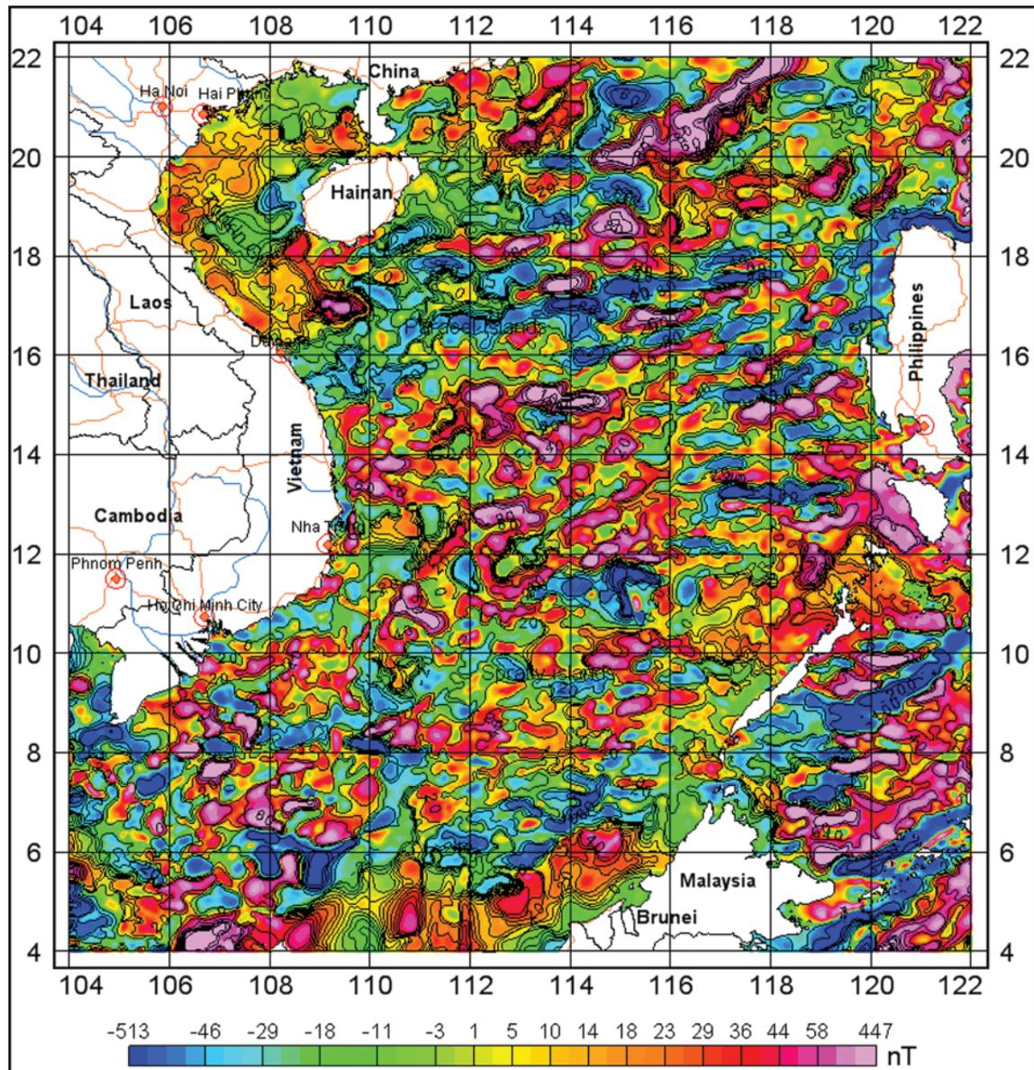
Fig. 2. Magnetic anomaly  $\Delta T_a$ .
