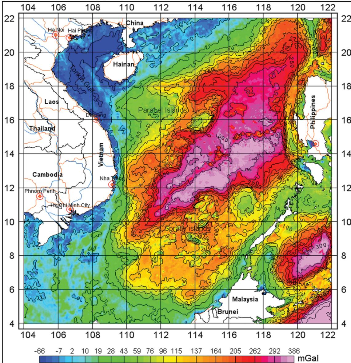
Fig. 1. Complete Bouguer gravity anomaly.
