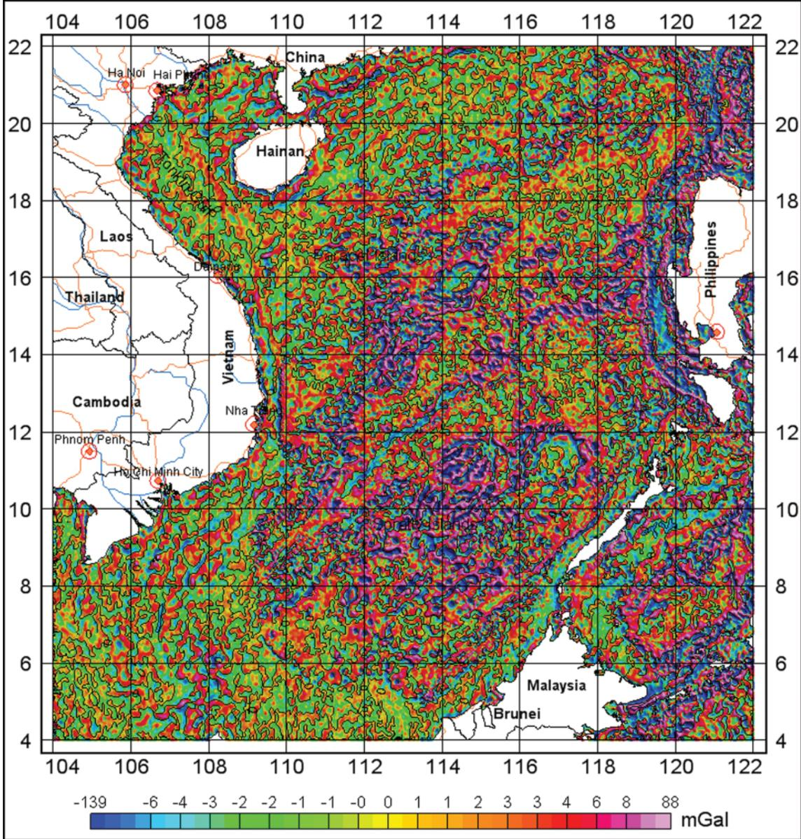
Fig. 5. Residual gravity anomaly at filtering wavelength  $\lambda = 50$  km.
