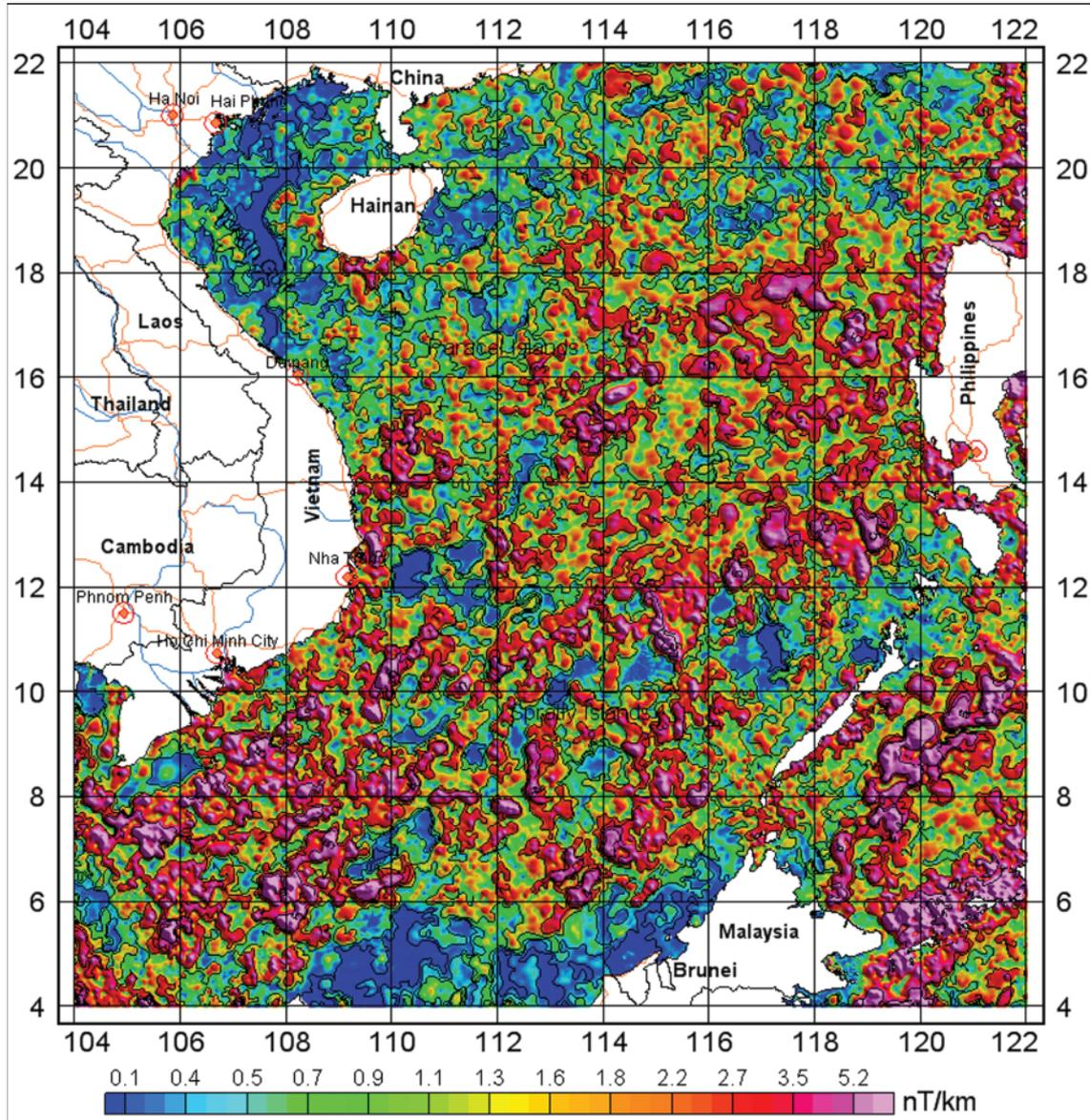
Fig. 8. 3D total gradient of magnetic anomaly.
